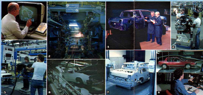
1. Computers aid in design and manufacture. 2. Robogate body framing. 3. Precision check of all body parts. 4. Worker team. 5. Instrument panel checking station. 6. ELPO bath of rust-resistant primers. 7. Master body cube with precision scanner. 8. Wind tunnel.
